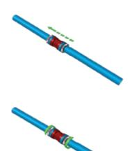
Align the two pipes and slide the fitting until the reference marks are visible on both sides.
