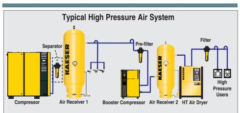
**Note:** All components must be properly pressure rated. Schematic does not show recommended accessories such as sequencers, drains, flow controller, or condensate management system. \* For compressors without an integrated moisture separator.
