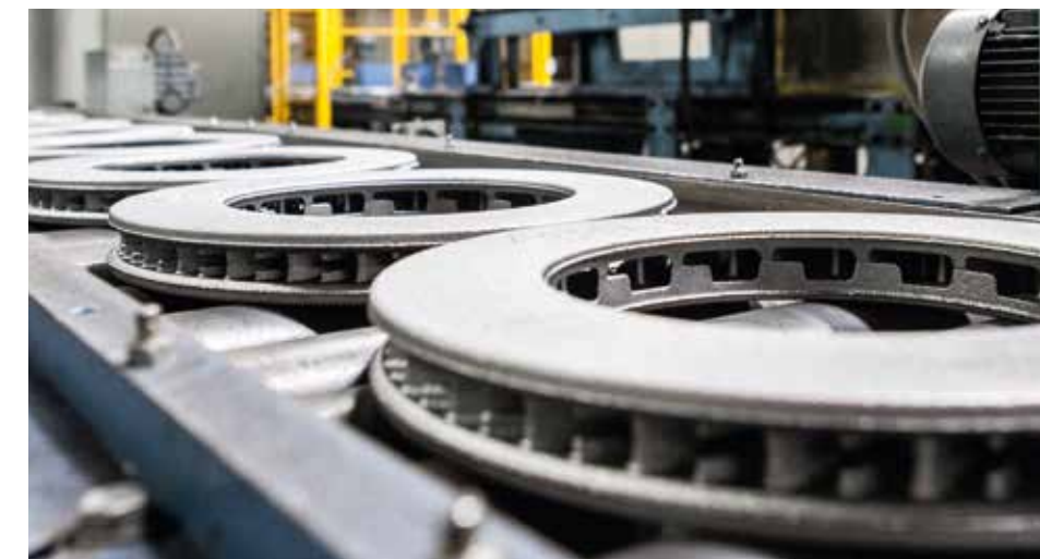
Raw friction rings roll off the production line
