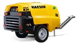
The M30PE delivers 100 cfm at 100 psi with a compact, low emission design.
