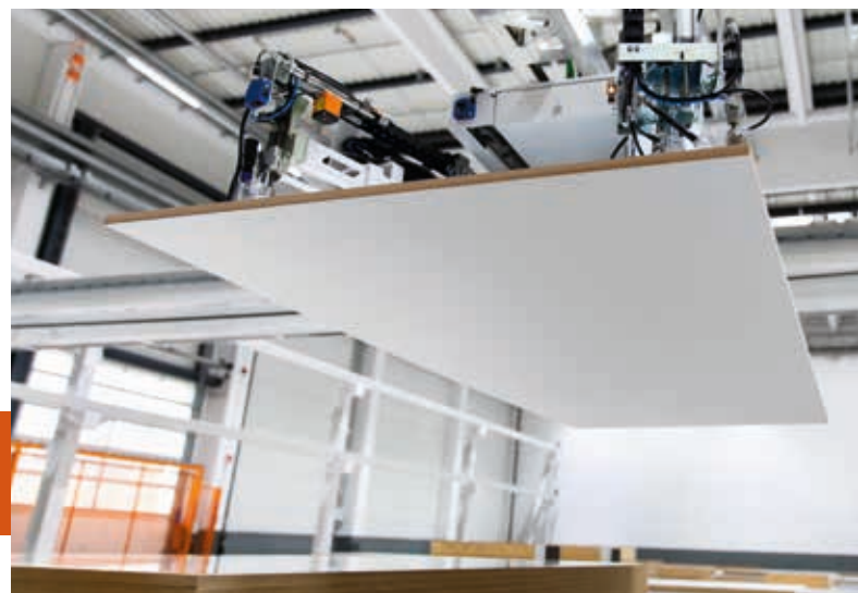
Compressed air is required for the suction machines that are used to lift large production pieces (via the Venturi principle).
