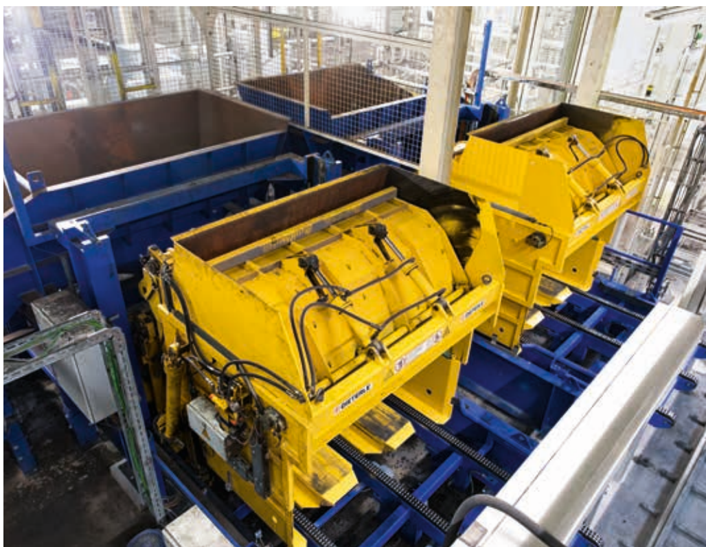
Preparation and charging for the coating of pourable bulk materials takes place in these lifting-and-tilting devices (drum processing).
