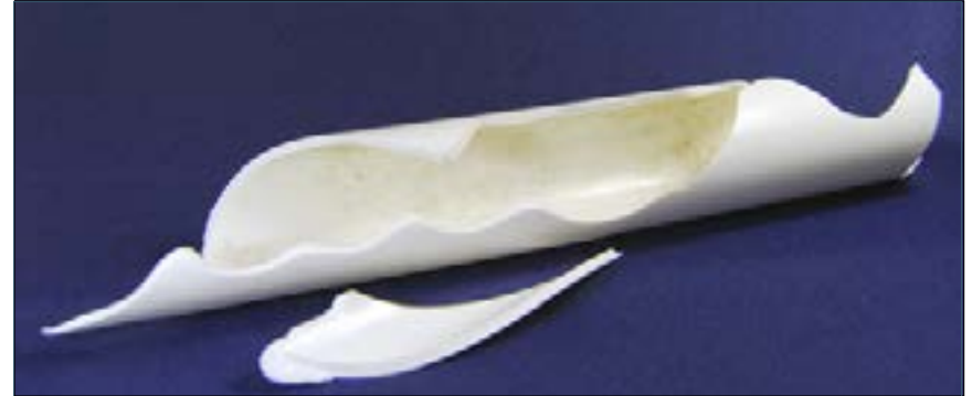
Burst PVC piping from a compressed air installation.
