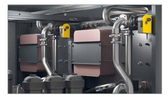
The integrated system comprised of the heat exchanger, thermostatic valve, and complete pipework requires no additional space around the compressor and can recover up to 72% of the overall power consumption of HSD compressors by utilizing the heat in the oil.
