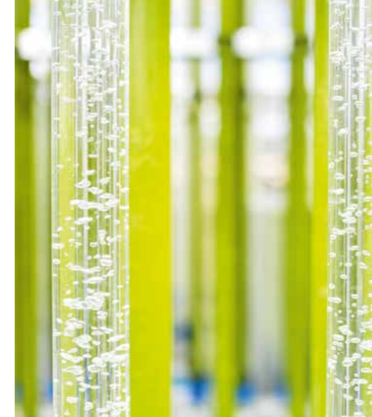
The main components of the system are long arrays of 20 foot tall, interconnected glass tubes.
