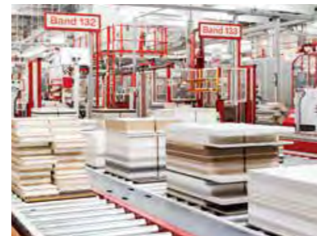
Compressed air is needed at every production stage: transportation of the wood panels shown here.
