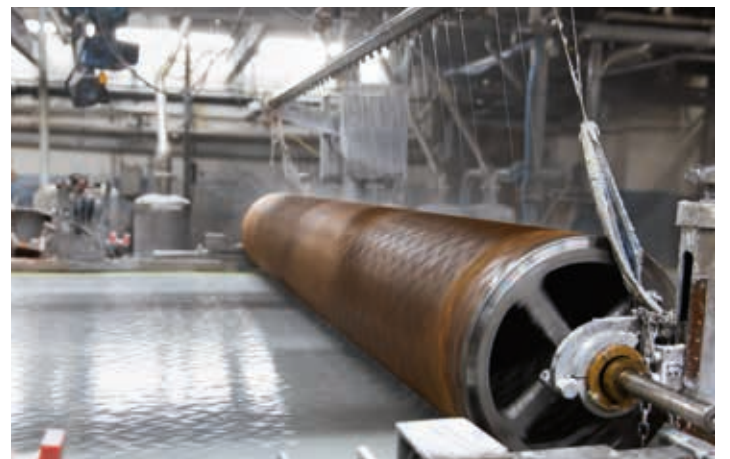
Watermarked paper is produced with the help of so-called dandy rolls.
