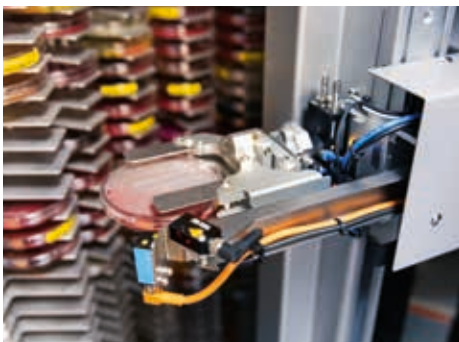
The compressed air performs a wide range of tasks in the large laboratory. Here with automatic handling of the Petri dishes...
