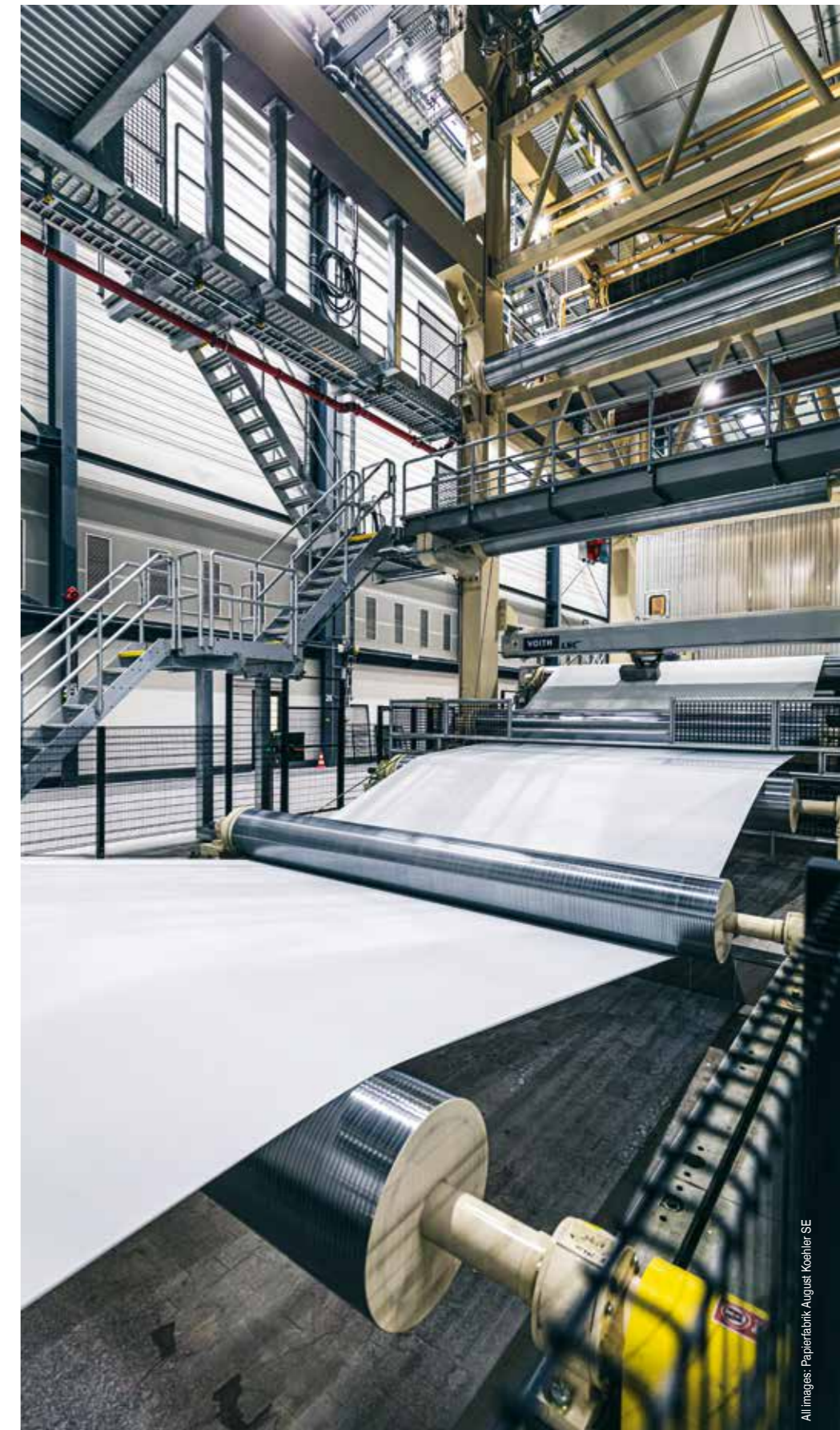
The paper machine known as PM 8 applies coatings to the paper that provide it with properties up until now only associated with plastics and composites.
