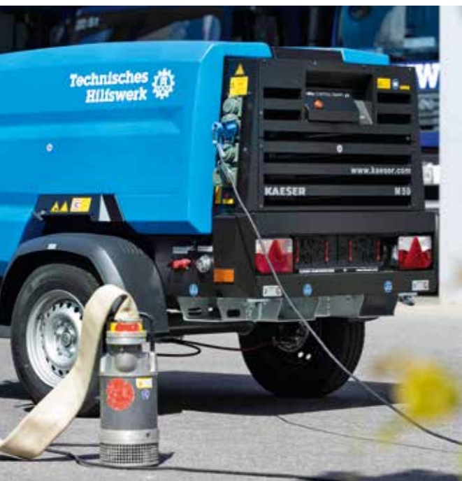
The new, road-going M59PE portable compressor is equipped with robust wing doors constructed of roto-moulded polyethylene.
