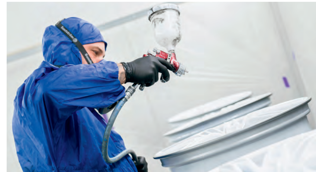
Compressed air is also used to power the paint spraying equipment.
