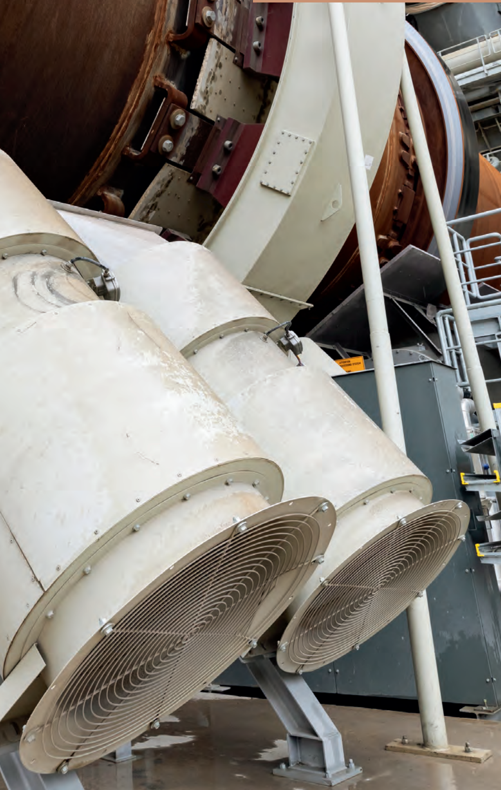
Lepol kiln with conveyor drive and shell cooling fans.
