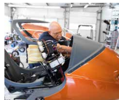
Final cockpit assembly: installation and connection of the aircraft’s avionics equipment.
