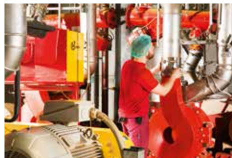
Compressed air is needed in every step of product processing. Shown here: material conveying.
