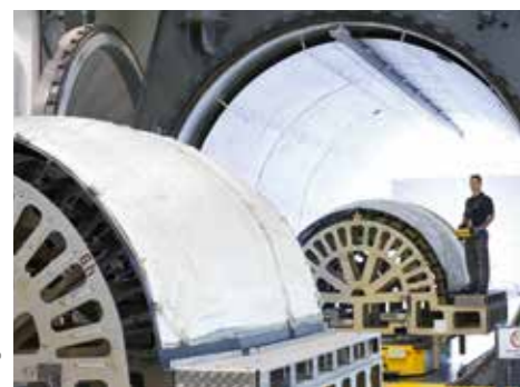
The engine nacelles are hardened in the autoclave to attain their final material characteristics.
