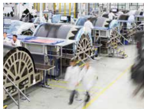
Up to 1000 or more layers of carbon composite material are combined to produce engine nacelles.
