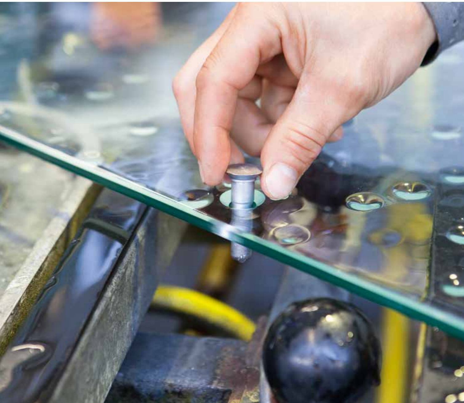
Drilling for hardware and other cutouts comes before the tempering process
