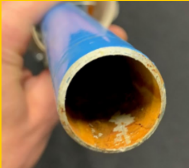
Left: aluminum piping with rust and scale after one year of operation.
