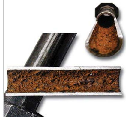
This actual cutaway of black iron compressed air piping shows typical contaminant build up and flow restriction after just a few years of operation.
