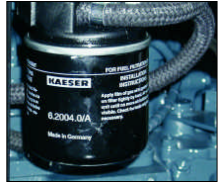
Inspect the compressor lubricant filter and change regularly.
