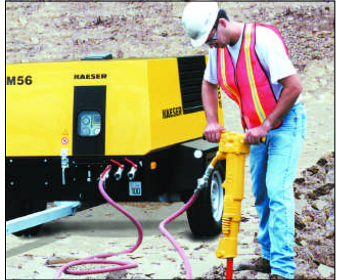
Compressor maintenance can be divided into seven sub-assemblies: pump or airend, drivetrain, engine, chassis, lubricants/fluids, filters and radiator.
