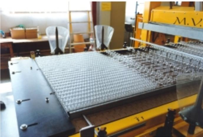
Vacuum is used for handling, transport and packaging of the glass vessels.
