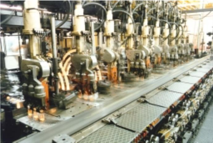
All kinds of hollowware are produced on the 40 individual operating stations with the help of compressed air.
