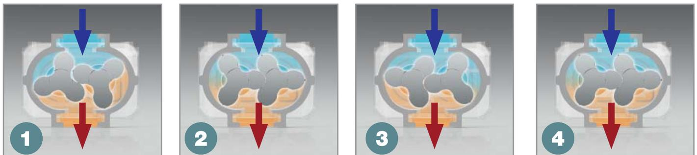
Image 1: Pressure increasing—the images show the cross-section flow chamber of Kaeser's rotary lobe blower block.
