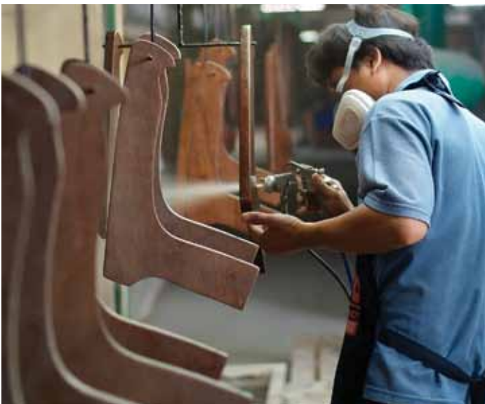
FIGURE 1: Woodworking shops are part of the unique segment of smaller compressed air system users that often need larger volumes of higher quality air for applying high quality finishes.
