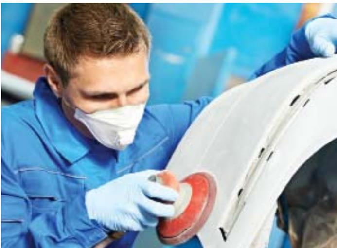
FIGURE 1: Collision repair shops are unique in the automotive service industry because they often need larger volumes of higher quality air for body work (shown here) and applying high quality automotive finishes.
