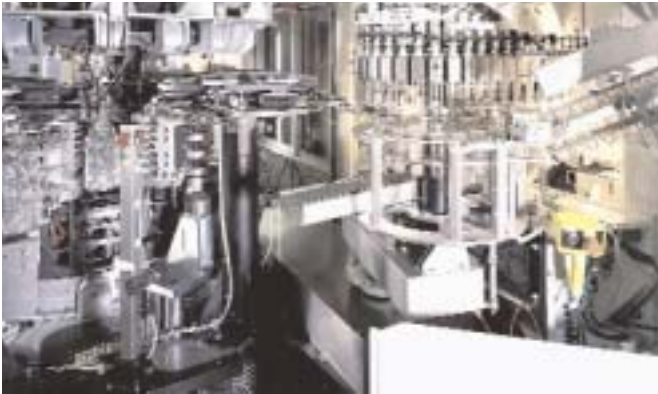
Fig. 3: Blow mould machines with preform feed lines and blow mould units.
