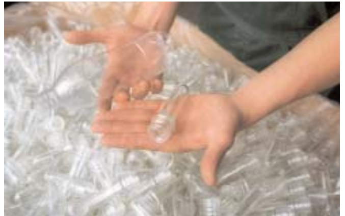
Fig. 2: The "preforms" are blown up to size as finished PET bottles in the blow mould machines. (Krones works photo)
