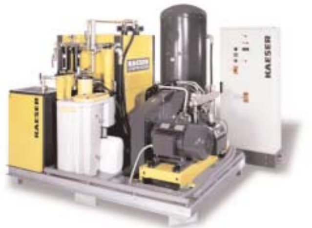
Fig. 5: A compressed air package supplying air to the blow mould machines. The package illustrated consists of a rotary screw compressor (low-pressure stage, rear left), a booster (high-pressure stage, front right), an air receiver (centre rear), control cabinet (rear right), and an Aquamat condensate treatment unit (centre front). The package can be made up of correspondingly more compressors, depending on requirements.
