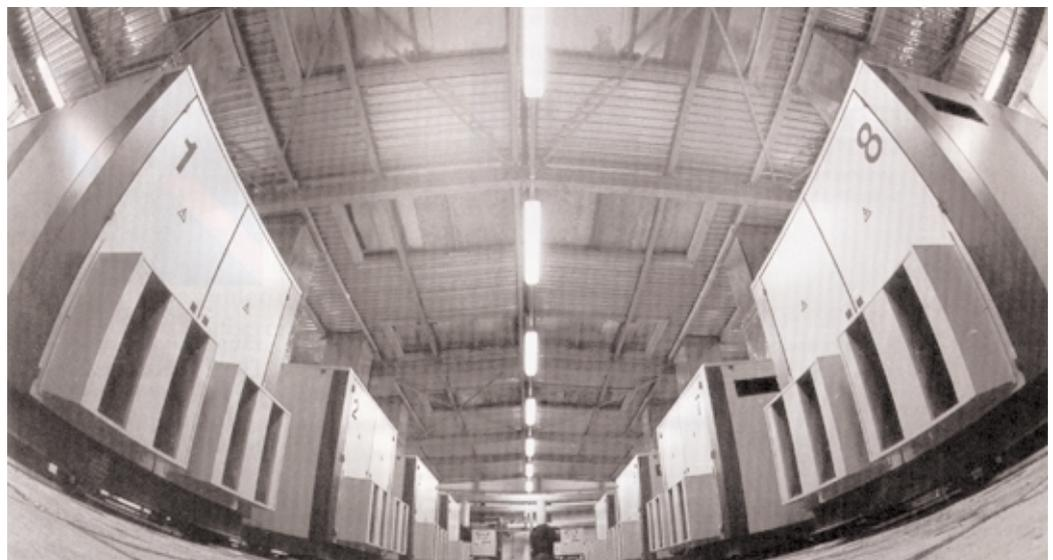
**Water-cooled machines must also be properly ventilated to dissipate radiated heat.**
