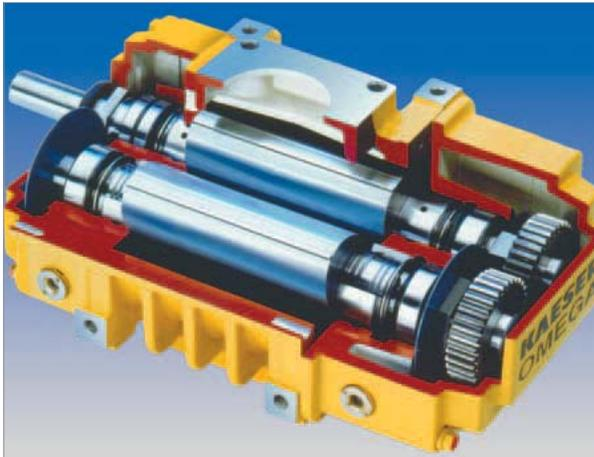
Rotary-lobe blowers are positive-displacement machines delivering constant volumes at variable pressure. Positive-displacement blowers are variable over a wide range of speeds and the power requirements are almost
