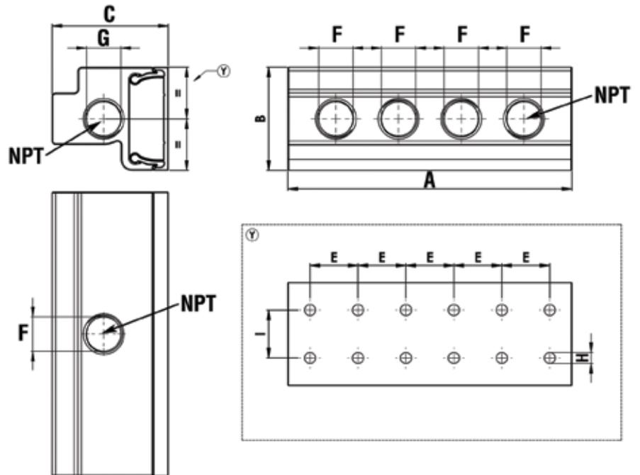
**MOUNTING HARDWARE NOT INCLUDED.** Manifold ships as shown without plugs.
