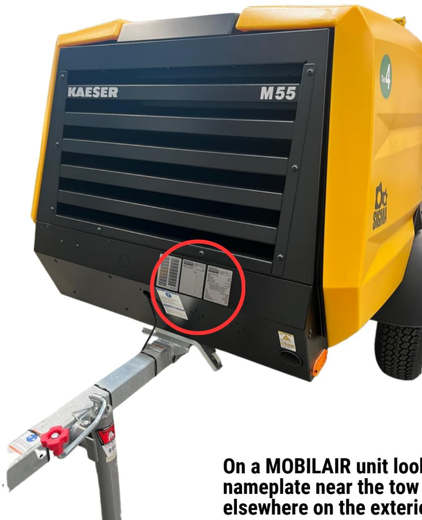
On a MOBILAIR unit look for the nameplate near the tow bar or elsewhere on the exterior body.
